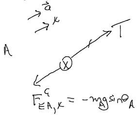
(c) Write Newton's second law,  $ma_x = \sum F_x$ , separately for each of the blocks. Since the cable stays taut, ax is the same for both blocks.
