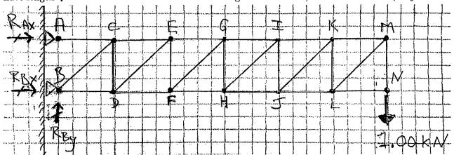
(a) Using the moment equation for the truss as a whole about joint B, determine the horizontal support "reaction" force  $R_{Ax}$ . What does the sign of your answer imply about the direction that this support force actually points?
