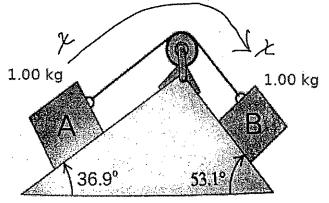
(b) Draw a Mazur-style free-body diagram (FBD, not EFBD) for block A, and draw a Mazur-style FBD for block B. Be sure to indicate, adjacent to each FBD, the direction of acceleration for the corresponding block.
