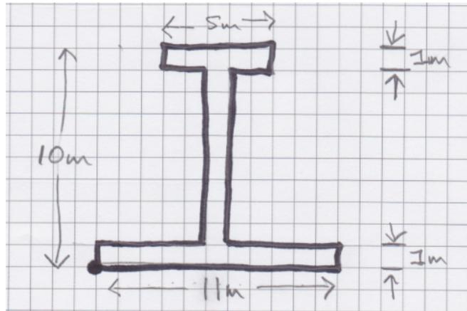
3. Find the centroid of the enclosed area shown below. Take the bottom-left corner of the enclosed area (where the large dot is drawn) to be the origin  $(0,0)$  of the coordinate system. The side of each square on the graph paper represents 1.0 m.
