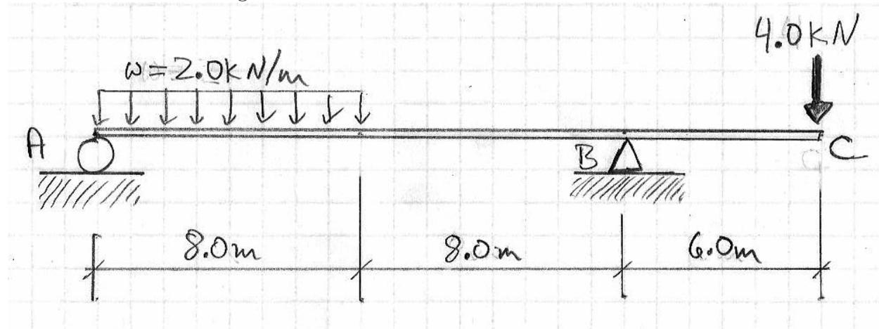
(a) Find the support forces  $A_y$ ,  $B_x$ , and  $B_y$  exerted on the beam by supports A and B.
