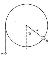
**XC8.** Optional/extra-credit. The right figure above shows a massless wheel of radius R, mounted on a frictionless horizontal axle. A point mass M is glued to the edge of the wheel, and a mass m hangs from a string wrapped around the perimeter of the wheel. (a) Write down the total PE of the two masses as a function of the
