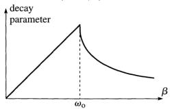
Figure 5.13 The decay parameter for damped oscillations as a function of the damping constant  $\beta$ . The decay parameter is biggest, and the motion dies out most quickly, for critical damping, with  $\beta = \omega_0$ .
