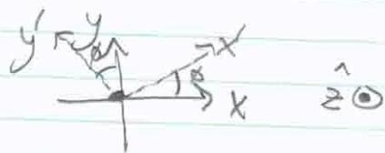
$$x' = x \cos\phi - y \sin\phi \quad y' = x \sin\phi + y \cos\phi \quad z' = z$$
