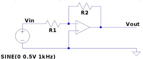
Now choose resistors for a gain of -10. Again, try 1 V<sub>pp</sub> inputs, and look at V<sub>out</sub>. What happens when you try a 5 V<sub>pp</sub> input? Now reduce the amplitude to 0.1 V<sub>pp</sub> sine waves and try increasing the frequency. Notice that the ideal behavior breaks down once you get up beyond a few hundred kHz — you can look at the opamp's data sheet if you're curious. (We'll discuss opamp real-life limitations next week.)
