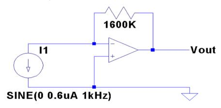
The idea, if all goes well, is for you to drive an LED (protected by a resistor) with the function generator, and then to detect that light with the photodiode, whose signal you will amplify and display on the scope. A rough illustration is shown below — though the exact resistor values will probably need to be adjusted.
