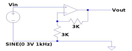
Now insert your non-inverting amplifier where the inverting amp was before (and where the follower was before that). What are  $V_{b1}$  and  $V_{b2}$  in this configuration? What do you infer about the input resistance of the non-inverting amplifier circuit?
