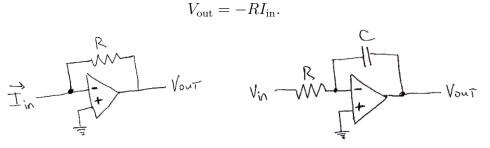
The next application (above, right) is called the **opamp integrator.** By Rule #1,  $V_{-} = 0$ , so the current flowing to the right through R is just  $I = V_{\rm in}/R$ . By Rule #2, current I must continue to the right through C, since negligible current flows into the opamp inputs. With the left side of the capacitor fixed at  $V_{-} = 0$ , the result of current I flowing through C from left to right is  $C \, dV_{\rm out}/dt = -I = -V_{\rm in}/R$ , so
